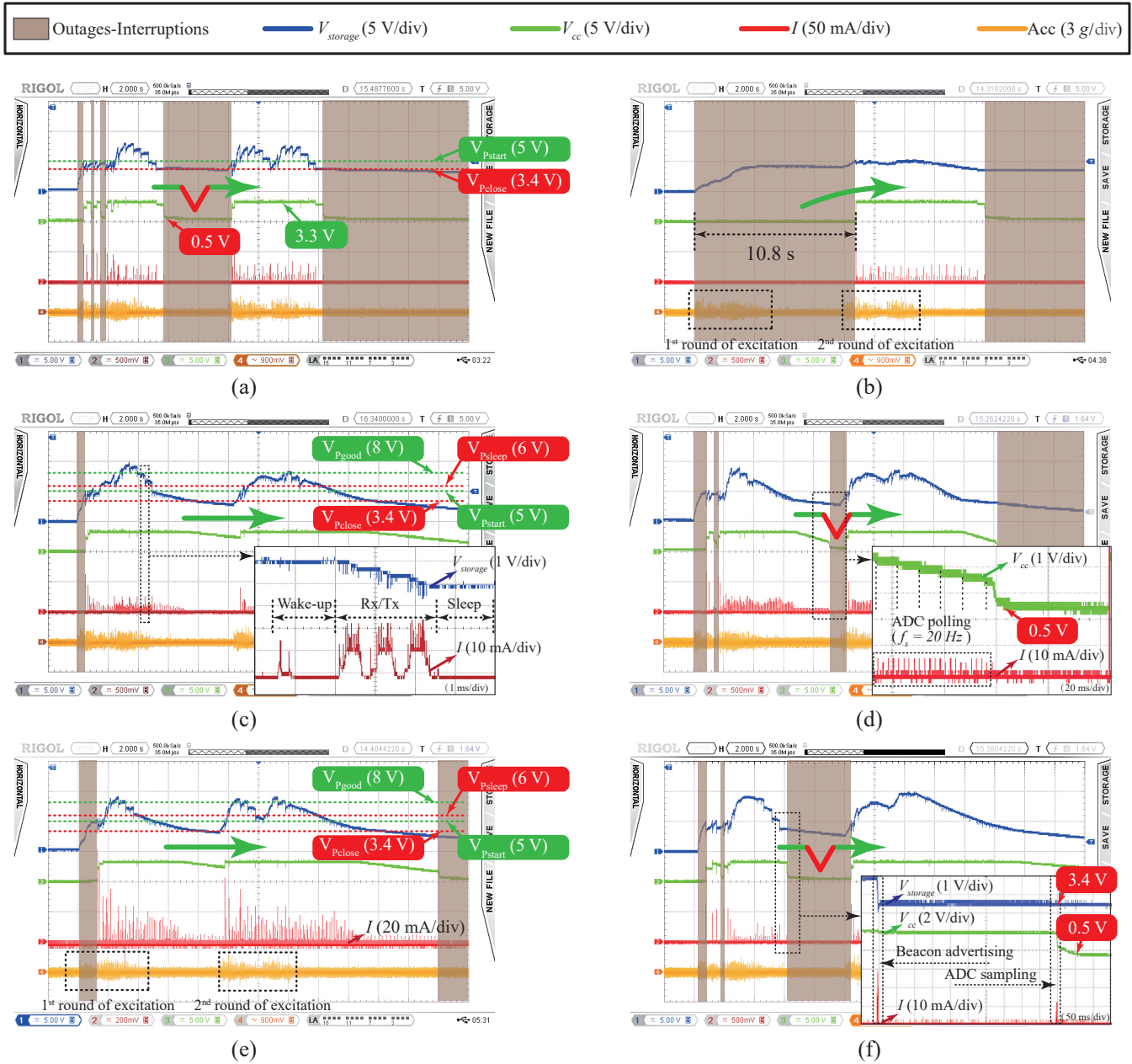
Fig. 6. Waveforms of the vibration-powered temperature sensor prototype with three different power solutions: UVLO (a, b), PID (c), and APC (d-f). (a) Startup with outage using a small storage (10 \mu F). (b) Success but slow startup without outage using a large storage (100 \mu F). (c) Execution without outage using energy indicating interrupt signals. (d) Startup with outage due to over-sampling ( f_s = 20 Hz). (e) Execution without outage using ADC polling check ( f_s = 4 Hz). (f) Execution with outage due to under-sampling ( f_s = 0.5 Hz). The frequency of the BLE Beacon advertisement is 2 Hz. (c) - (f) use a small storage capacitor (10 \mu F). V_{Pstart} and V_{Pclose} are fixed thresholds, while V_{Pgood} and V_{Psleep} are tunable according to the most energy-consuming atomic operation.
